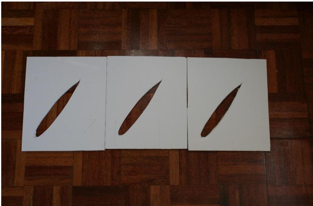
When placed together this gave enough depth for the float to sit comfortably in the foam board stack (expert advice has since told me the plane should be sitting higher in the water and the stabilising floats should be clear of the water).
